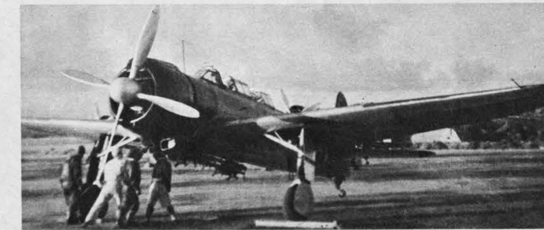
DIHEDRAL from the wing roots on Jill 12 should prevent confusion with Kate 12. With their carrier fleet below full strength, the Japs have been using single-engine torpedo planes from land bases.
